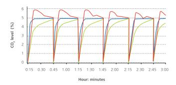
Precisely-tuned sensor and software result in fast recovery of CO, without overshoot. This ensures uniform CO, levels even with frequent incubator door opening.
