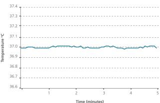
Different lines represent different sensor positions inside the chamber. Esco CelCulture® has uniformity variance of less than ± 0.5°C which means all the samples are evenly heated.\*
