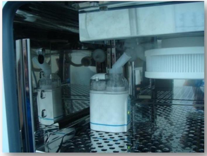
**Figure 1. Smoke test to checking the airflow pattern**
