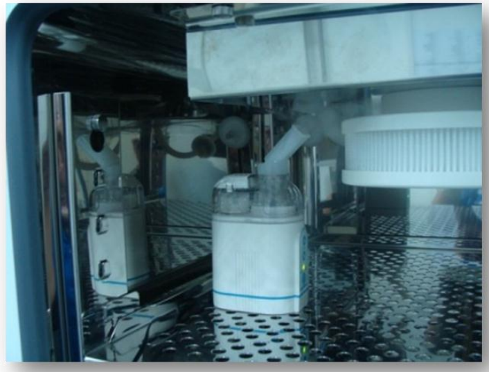
Figure 1. Smoke test to checking the airflow pattern
